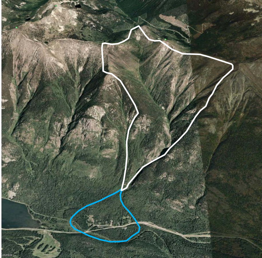
Figure F-2. A Google Earth image of a typical steep creek watershed (Charlie's Creek) located near Nakusp in the RDCK. The approximate watershed and fan boundary are outlined in white and blue, respectively.
