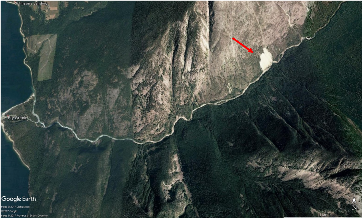
Figure F-7. Example of evidence for recent landslide activity within the basin of Fry Creek Fan No. 101.
