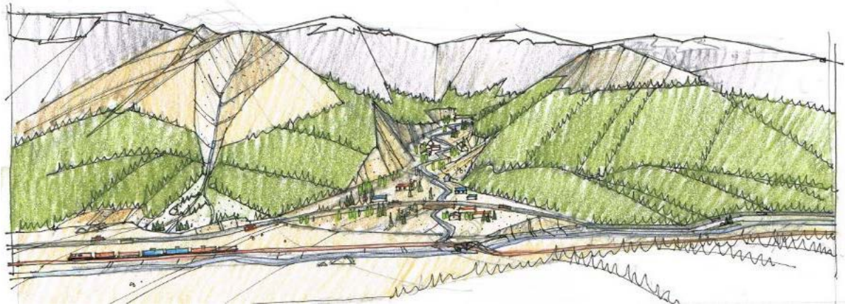
Figure F-3. Typical steep and low-gradient fans feeding into a broader floodplain. On the left a small watershed prone to debris flows has created a steep fan that may also be subject to rock fall processes. On the right a larger watershed prone to debris floods has created a lower gradient fan. Development and infrastructure are shown to illustrate their interaction with steep creek hazard events. Artwork: Derrill Shuttleworth.
